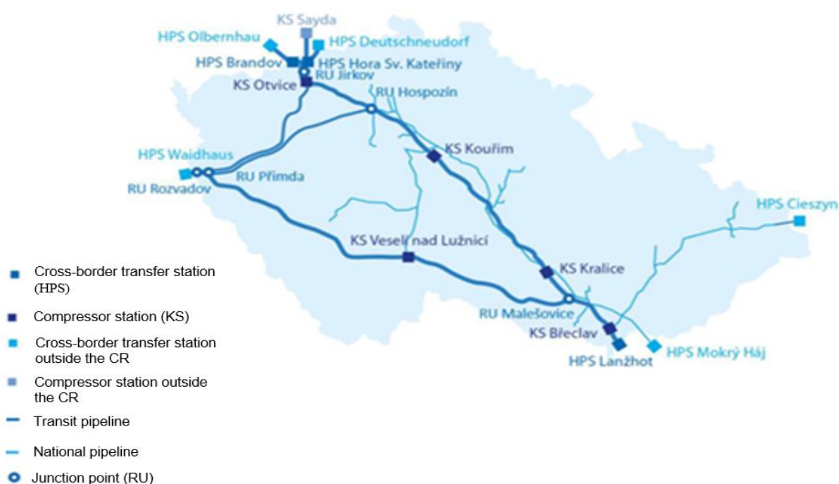
Figure 5 Structure of the transmission network
